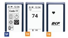
If you press any button, the heart rate display will be activated for another 10 seconds 20. If the connection (temporarily) fails, then the heart symbol will remain empty 21. Heart rate values can be recorded for a maximum of approximately 30 hours. After this point, the earliest recorded values will be overwritten.
